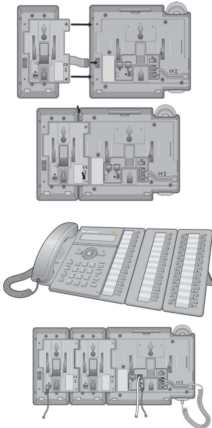
Figure 6.1.4.3-1 LIP-8000 DSS Installation
