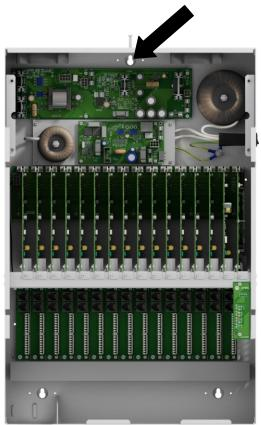
4. Screw the server and mark two bottom holes. Drill the points marked on the wall and fasten the server also with the bottom two screws.
